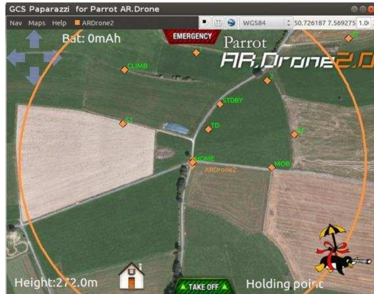
Figure 1: View of the Ground Control Station of Paparazzi for the Parrot AR drone 2. The overlays include current information of the drone's state such as its height, controls such as the home-button, and the waypoints in the flight plan.
