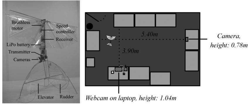
Figure 4: **Left:** the 15-gram ornithopter used for the height control experiments. **Right:** map of the room used in the flight experiment. The pilot only controls the rudder of the ornithopter; the height is controlled autonomously. The ornithopter is filmed from two viewpoints: by the webcam of the laptop and the camera used in the previous experiment.
