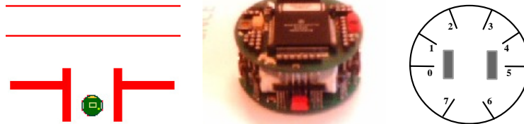
Figure 1: Left: experimental task. Right: the Khepera robot with eight infra-red distance sensors.
