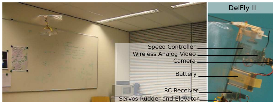
Figure 1: The 16-gram, 28 cm wing span flapping wing MAV DelFly II during an obstacle avoidance experiment with monocular vision. The inset shows the top of the DelFly’s body with its electronic components.
