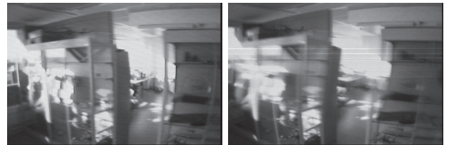
Fig. 7. Two subsequent images in a video made onboard the DelFly II with deformations caused by the combination of the flapping frequency of the DelFly and the line-by-line recording of the camera.
