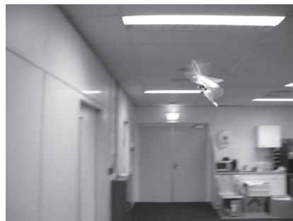
Fig. 1. External image of the 16-gram flapping wing MAV DelFly II during the obstacle avoidance experiment.
