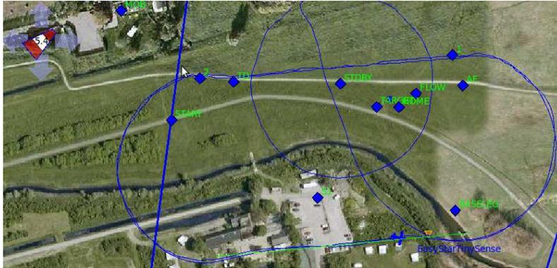
Figure 16: Part of the flight trajectory as shown on the Paparazzi ground control station. The MAV is flying along the green line in the direction of the orange ‘carrot’.
