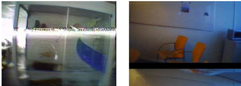
Figure 1: Example noisy / bad images. Left: WiFi transmits on the same frequency as the analog camera and introduces noise especially in a horizontal band. Right: the receiver loses track of the start and end point of the image.
