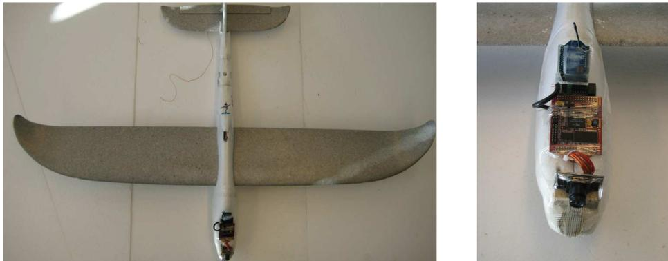
Figure 15: Left: Fixed wing MAV used for the real-world experiments. Right: modified Surveyor SRV-1 BlackFin camera mounted on the nose.
