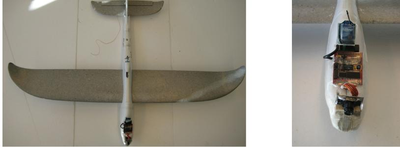
Figure 13: Left: Fixed wing MAV used for the real-world experiments. Right: modified Surveyor SRV-1 BlackFin camera mounted on the nose.
