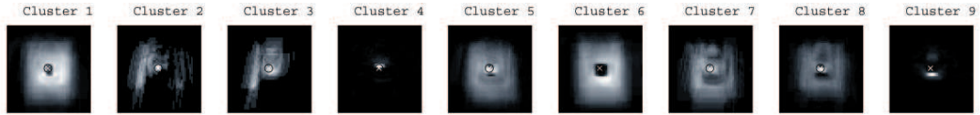
Figure 5: Distribution of the nine input clusters relative to the target location. The center of the license plate is in the center of each image and is indicated by a white cross surrounded by a black circle. For each coordinate, the light intensity is proportional to the frequency of occurrence of each cluster. These results were obtained with a sampling window size of one sixth of the image width.
