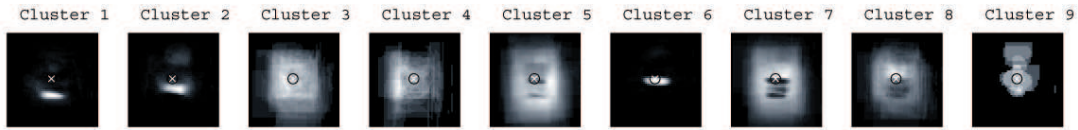
Figure 3: Distribution of the nine input clusters relative to the target location. The center of the license plate is in the center of each image and is indicated by a white cross surrounded by a black circle. For each coordinate, the light intensity is proportional to the frequency of occurrence of each cluster. These results were obtained with a sampling window size of one third of the image width.
